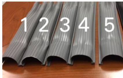
Torsion Source initially looked at astragal designed with a tapered web. The decision was made to modify the design and create a step in the webbing. This helped to give rigidity to the "T" areas. Testing was then conducted on samples in the new profile with the following variations in material (pictured in order
